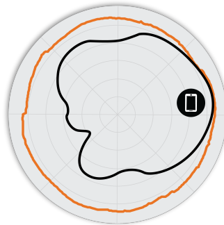
Figure 3. E510 5GHz Azimuth Antenna Patterns
