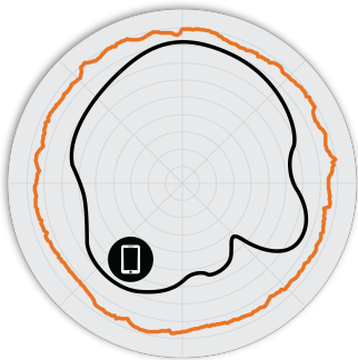
Figure 2. E510 2.4GHz Azimuth Antenna Patterns
