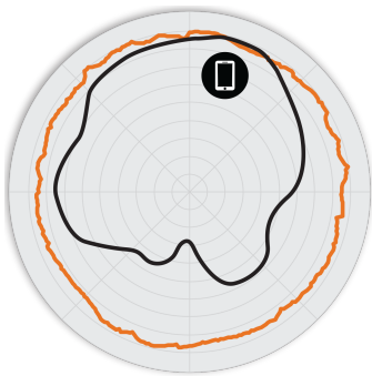
Figure 2. R730 2.4GHz Azimuth Antenna Patterns
