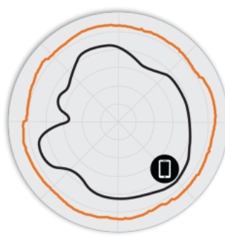
Figure 3. R730 5GHz Azimuth Antenna Patterns
